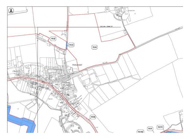
The update to the application would involve removing the on-road option for 132kV cabling which currently follows the section of adopted highway through Bishopton known as The Green and High Street. The proposed removal is shown on an indicative Red Line Boundary overview plan extract below. This land comprises part of plots 9/6 and 11/11 and the whole of plot 11/8 and is no longer necessary to guarantee delivery of the Proposed Development now that the Easement Option is secured.
